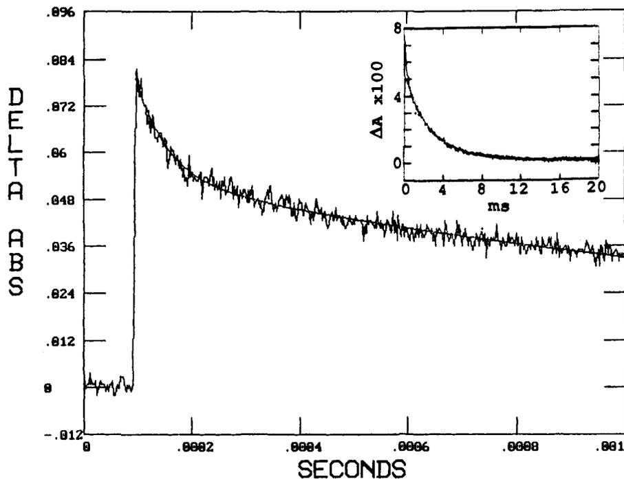
Figure 2. Transient absorbance at 460 nm in a solution containing 10  $\mu\text{M}$  covalent complex Zncyt/pc (derivative 5 from a column of CM52) in phosphate buffer of ionic strength 10 mM, pH 7.0, at 25  $^{\circ}\text{C}$ . The solid line is a biexponential fit. Inset: The same, over 0.02 s, to show complete recovery of the ground state.
