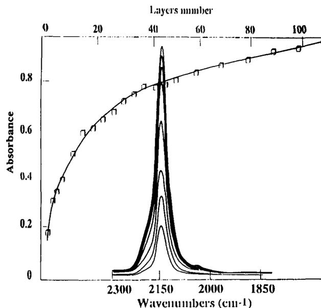
Figure 1. Absorbance bands  $\nu(\text{C}\equiv\text{N})$  as increasing number of layers are casted. In ascending order, 2, 4, 8, 20, 40, 60, 80, 100 layers (lower x axis). Upper axis: graphic representation of above bands as function of number of casted layers.
